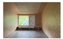
The members of St Martin's Scouts carried out the façade work and interior work, including the wall panelling with three-layer panels with acoustic perforations, themselves.
